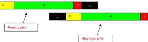
Considering that 1 hour of CAM programming can lead to approximately 3 hours of uninterrupted machining (set-up and turnaround included), it is desired to keep the scheduled machining time at the maximum.
